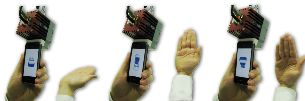
Figure 1: Using the pose of the flat hand behind the device to freely rotate a 3D object. A depth camera is used to determine the hand posture.
